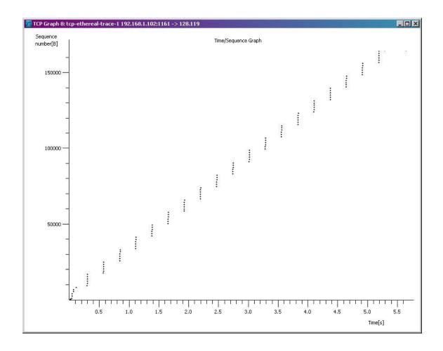
Each dot in this diagram represents a TCP segment that was sent, and the plot shows the sequence number of the segment in relation to the time at which it was transmitted. It is important to take
